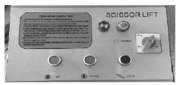
When the power supplied, turn the *POWER SWITCH* clockwise while the machine is on standby and an *INDICATOR* will show.
